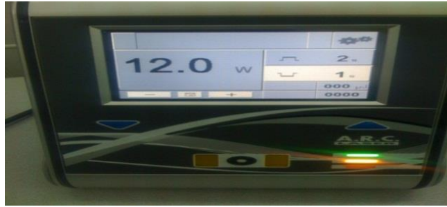
Figure (6): the laser system in action 12 watt pulsed waves 2 m sec intervals
